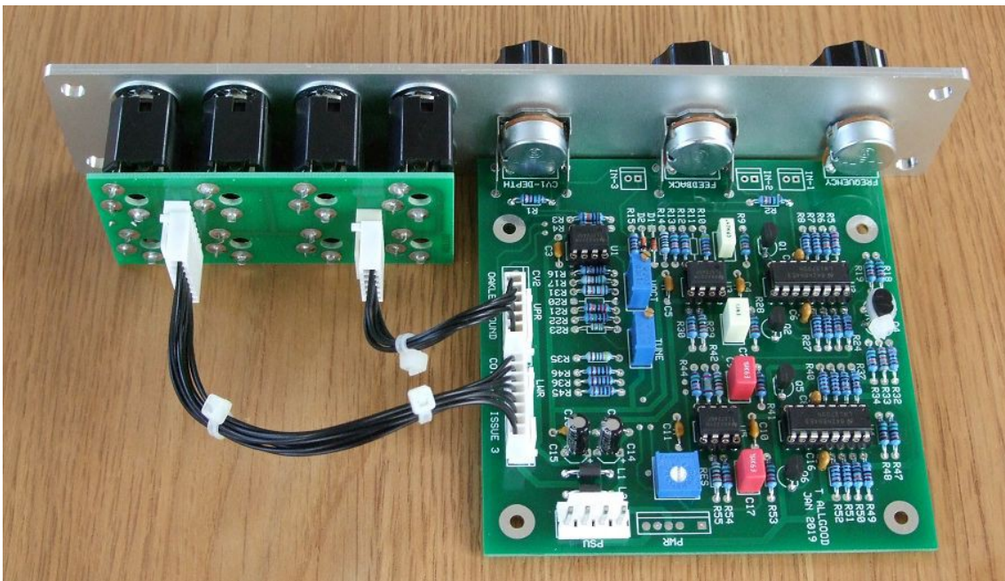
The issue 3 COTA behind a 1U wide MOTM format natural finish Schaeffer panel.
