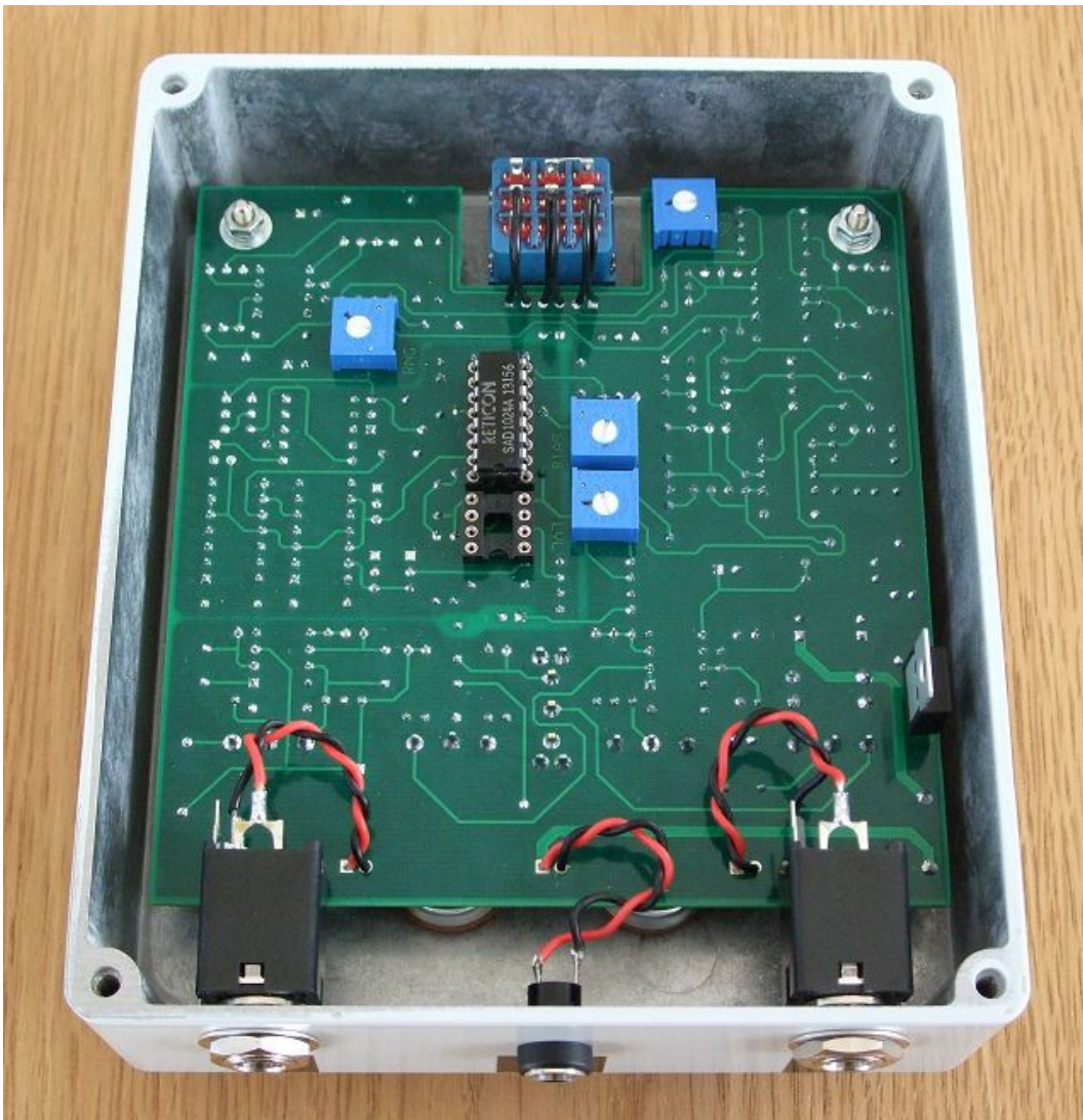
The guts of a completed Oakley Vintage Flanger. Since this particular unit was built to test both SAD1024 and SAD512D devices both 8-pin and 16-pin IC sockets have been fitted to the underside of the board.
