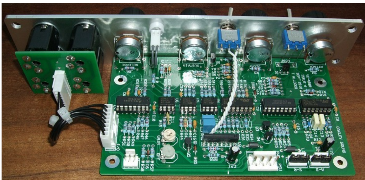
The issue 4 VC-ADSR/VCA board mounted behind a natural finish MOTM size Schaeffer panel. Note the two 0.1" KK headers on the lower right. These headers can be attached to the 1U Upgrade module to allow for full voltage control of the modules four parameters.
