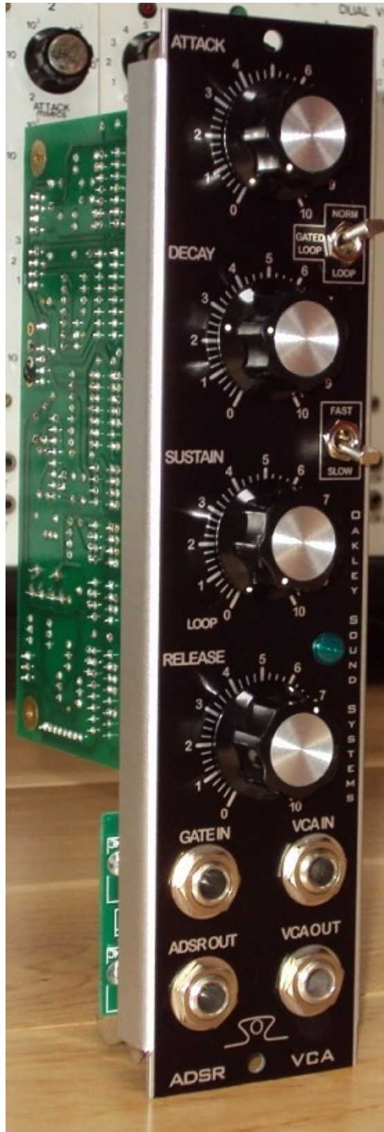
The single width ADSR/VCA module in Moog Unit (MU) compatible format.
