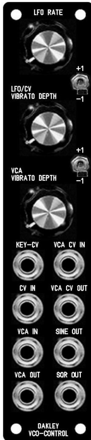
*The suggested panel for fitting to an Oakley modular system with the Oakley CV/gate bus. The twin keyboard control voltage (KCV) signals that this module generates are connected to the VCOs behind the front panel. If you do not have the facility for this you can make two of the front panel sockets carry the two KCV signals instead.*
