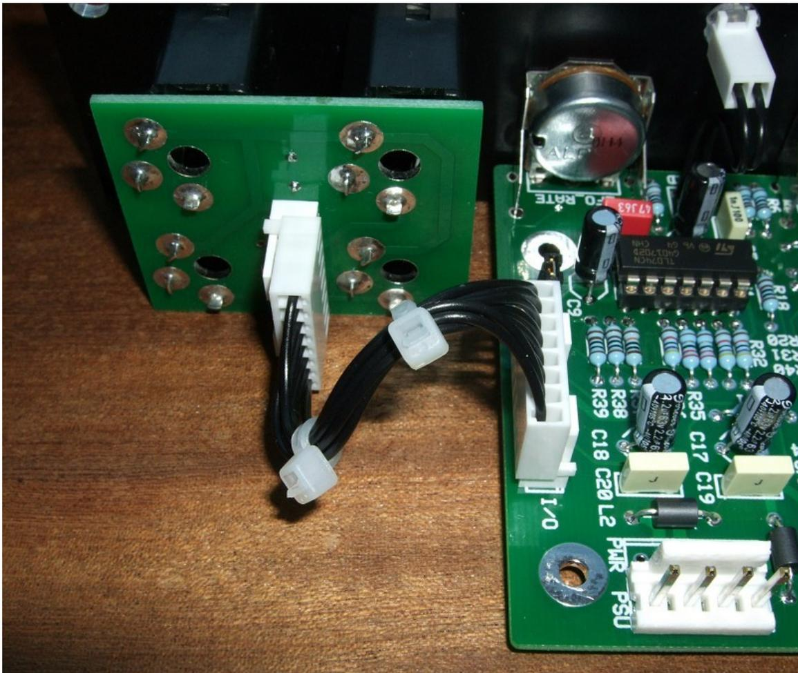
*The prototype Equinoxe unit showing the detail of the board to board interconnect. Here I have used the Molex KK 0.1" system to connect the Sock4 to the main PCB.*
