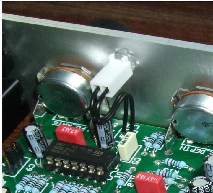
*Using a two way Molex KK housing to connect the bi-colour LED to the circuit board. The LED is held onto the panel with a clear Cliplite lens, or equivalent, available from various places.*
