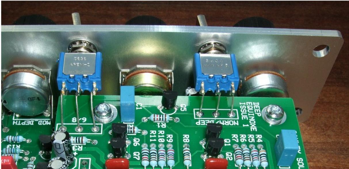
The switches are simply wired to the Deep Equinoxe board with stiff solid core wire although you can use multistrand hook up wire if you like. The solid core wire is looped around each switch lug and soldered in place. I recommend that the wire has some slack to allow the boards to flex a little.
