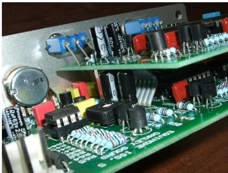
*The view between the two boards. Low profile electrolytic capacitors would probably have been better in this case as the two lower ones nearly touch the underside of the Deep Equinox board.*
