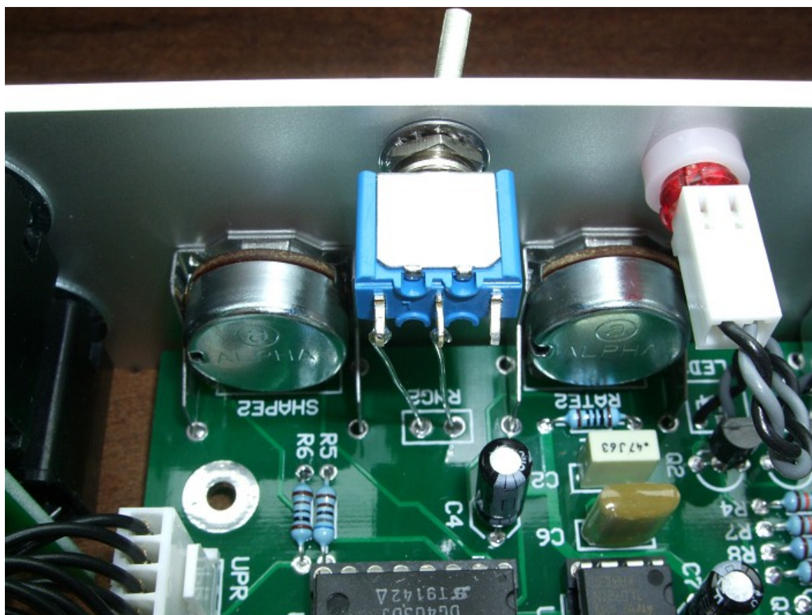
This is an Apem SPDT (on-on) toggle switch. Note that for both switches it is the lower two tangs of the switch that connect to the PCB.
