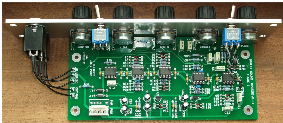
The prototype Overdrive-II module fitted to a natural finish Schaeffer MOTM format panel.
