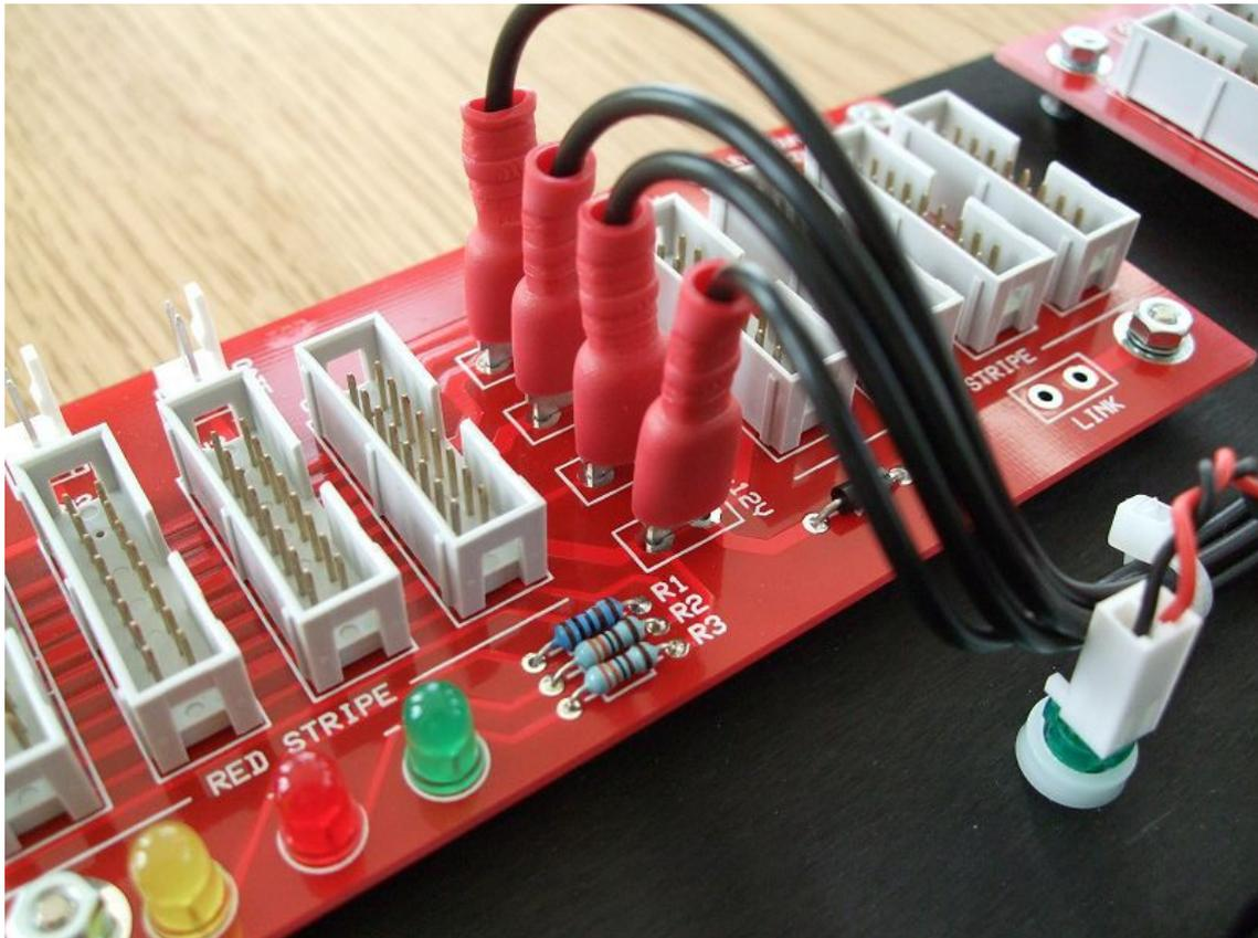
*Red faston connectors being used with 24/0.2 wire. Although I haven't done it here, colour coding your wires is a good idea.*
