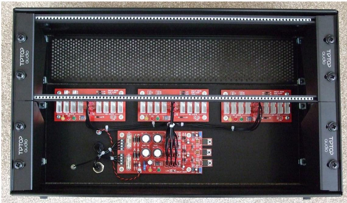
*An example 6U modular system case showing three Dizzy distribution boards fitted to a rear mounted 4U high blank 3mm aluminium 19" rack panel which also holds an Oakley Euro PSU and associating sockets and switches.*
