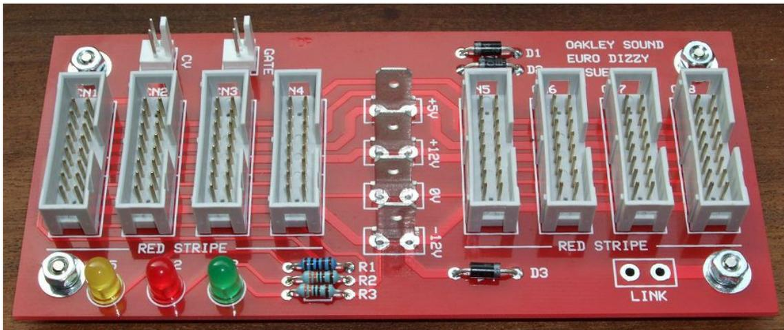
*A fully populated issue 1 Euro Dizzy board fitted with eight Oupiin 3012-16C00SYA headers and two Molex KK 0.1" headers for CV and gate. The link has not been soldered as there is no need to do so in this particular case.*
