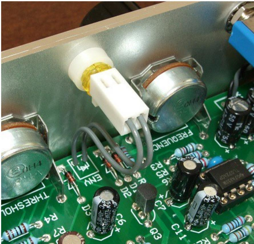
*All three LEDs can be wired in by using Molex KK 0.1" housings and solderless crimps. The LED clips used here are the low profile types with white securing rings.*
