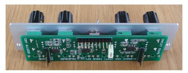
The pot board fitted to the front panel. Note that all the surface mount components are fitted to this side.
