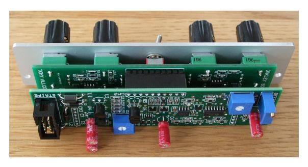
The module comprises of two circuit boards connected together with one 10 way 0.1" and two 6 way SIL headers and sockets.
