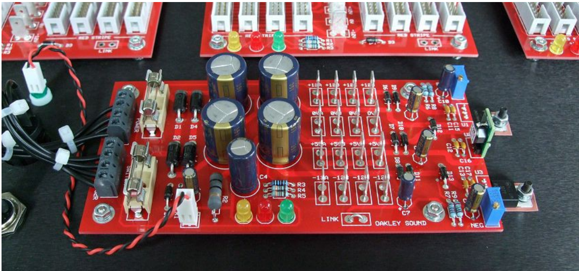
The issue 1 Oakley Euro PSU board with +5V DC-DC converter option fitted to a 4U panel awaiting connection to three Euro Dizzy distribution boards..
