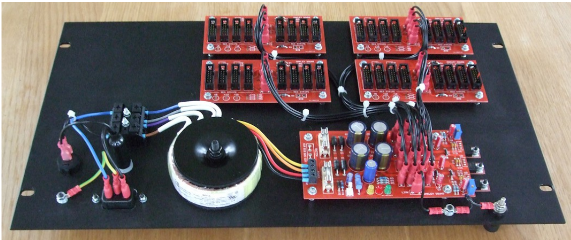
A standard 6U high 19" panel with a mains powered Oakley Euro PSU and four Euro Dizzy boards. Note the earth bond the left of the main power inlet, and the 0V bond and banana socket below the EPSU board.
