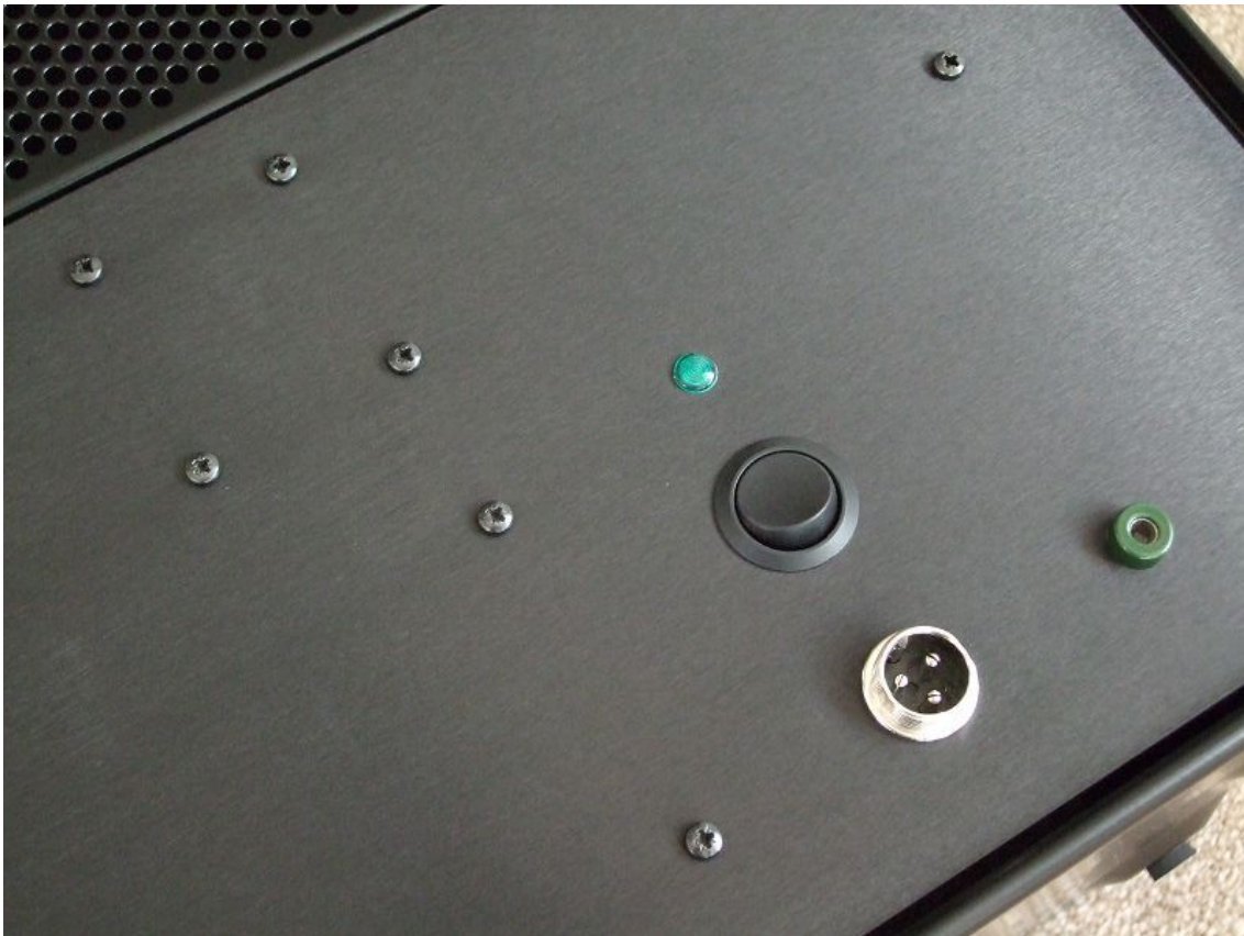
The additional 4mm socket to the right of the power inlet provides a way of connecting the 0V lines between cases.
