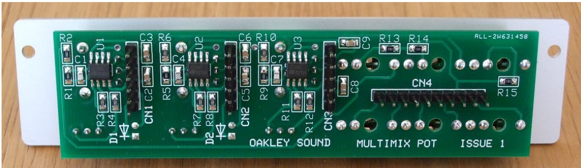
The top side of the pot board. The board is already fitted to the front panel. Note that all the surface mount components are fitted to this side. The pots and sockets cannot be seen as they are fitted to the underside of the board.
