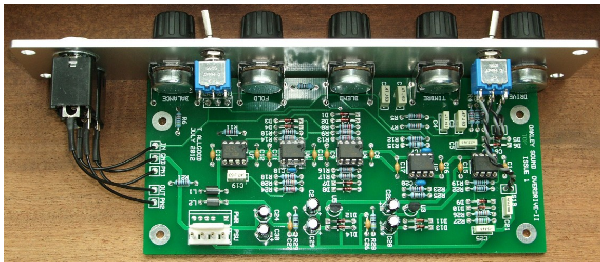
The original issue 1 Overdrive-II fitted to a natural finish Schaeffer MOTM format panel.
