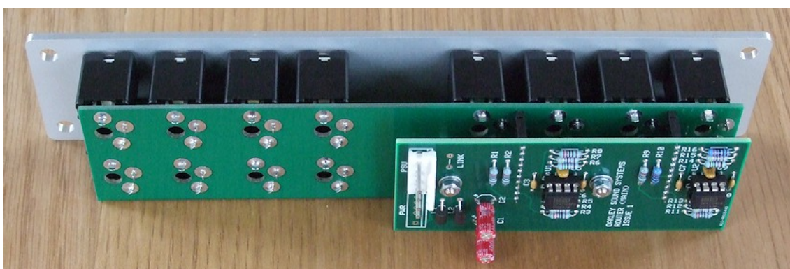
The issue 1 Oakley Router as a single width MOTM format module in a natural finish Schaeffer panel.
