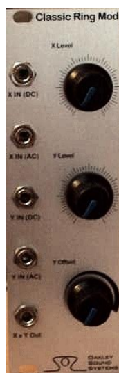
The current version of the Krisp1 Oakley Ring Mod. Older versions have only two input sockets and two switches.
