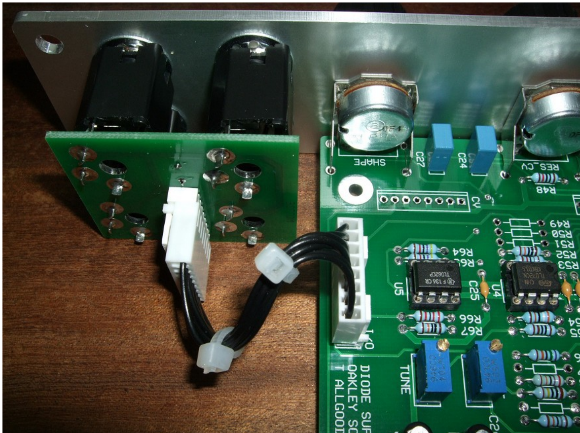
The prototype Diode Superladder filter core module showing the detail of the board to board interconnect. Here I have used the Molex KK 0.1" system to connect the Sock4 to the main PCB.
