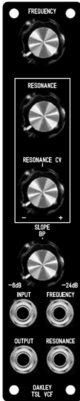
The suggested panel layout for the 1U filter core in MOTM format.
