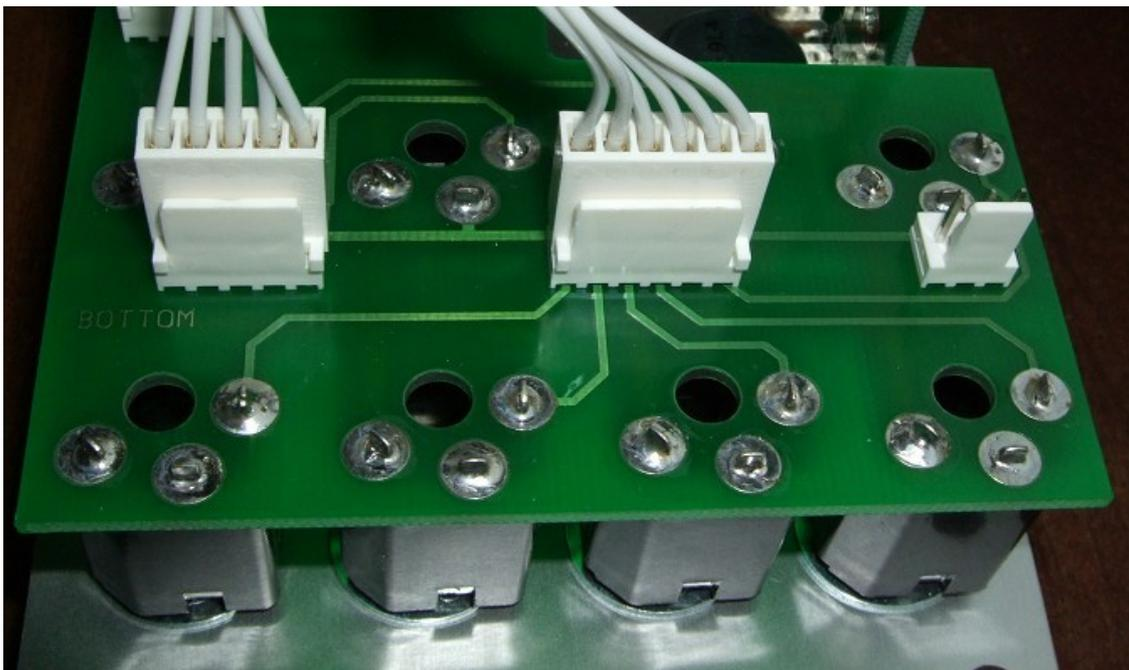
*There are four headers on the VCO module's socket board. Three of them will be fitted with connectors that go to other parts of the module. The Oakley Buss is the unconnected three way header on the right. If you are not intending to use it it should have a small two way jumper link inserted across pins 1 and 2. Pin 1 is the one furthest to the left and nearest the other big connector.*
